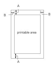
A The minimum top and bottom margins are 0.17 inch (4.2 mm).
